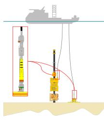
The Flint Subsea Kill Line Connector is installed on the end of a downline or jumper and provides protection against vessel drift or drive-off. It is a full-bore pressure balanced system suitable for operating in up to 10000ft water depth and pressures up to 15000PSI. Normal connection and disconnection is performed with the hotstab whilst emergency release occurs passively or actively via the Mid Line Weak
